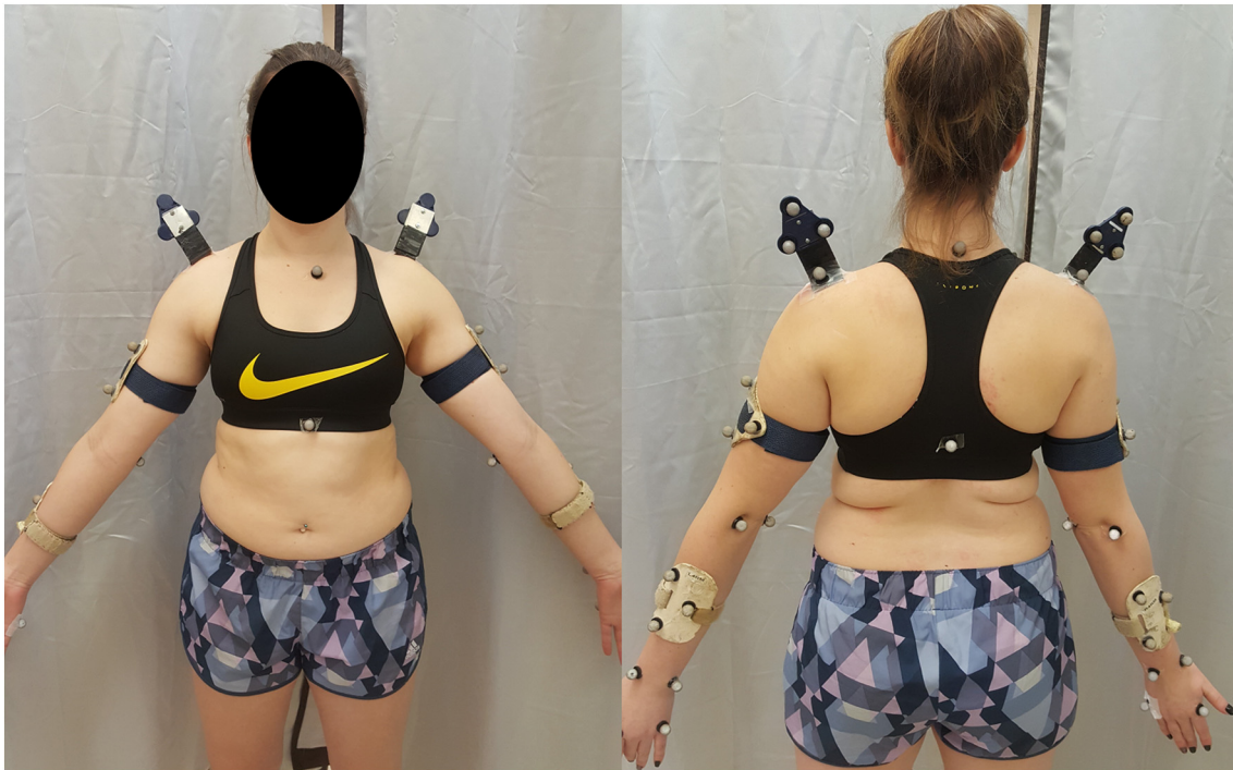
Fig. 1. Motion capture setup. Motion capture markers were placed over bony landmarks of the torso and upper extremity, with acromion clusters placed directly over the flat part of the acromion.
