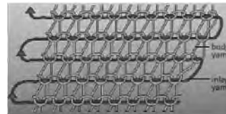
Inlay and body yarn in a flat knit garment
